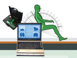
this it is possible to measure the pressure distribution of a cushion. A large number of pressure sensors are integrated into the mat and these measure the socalled interface pressure between the buttocks and the cushion.
